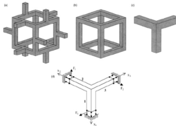
Fig. 2. Unit cell geometry and boundary conditions: (a) open structure; (b) simplified; (c) one-eighth; (d) under triaxial loads [2]
