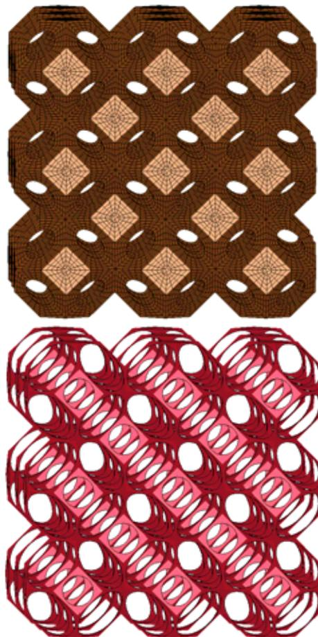
Fig. 7. Open cell foam microstructure models
