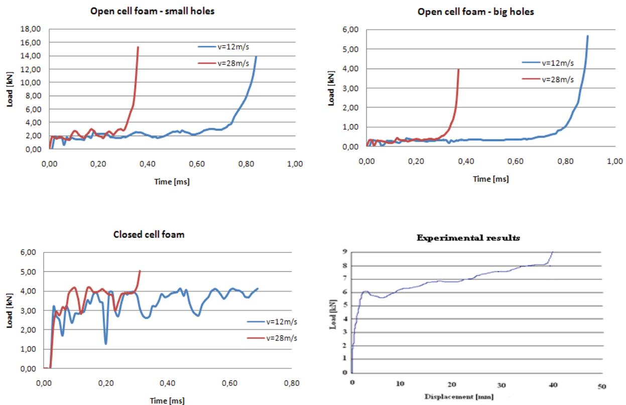
Fig. 8. Load- time charts for the numerical analyses and the experiment
