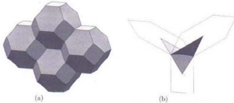
Fig. 1. Four cells in the Kelvin foam (a), and one fundamental piece (b), consisting of a fourth of one square and sixths of two hexagons, the region near a particular triple edge
