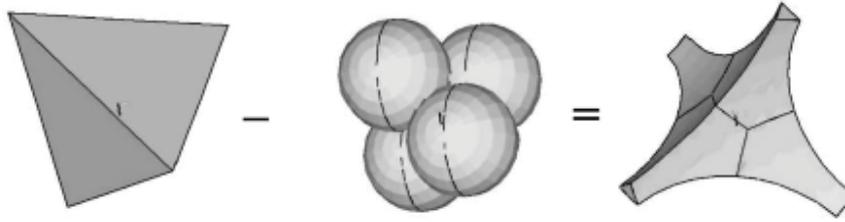
Fig. 3. A tetrahedron and spheres to generate a unit cell of a foam [3]
