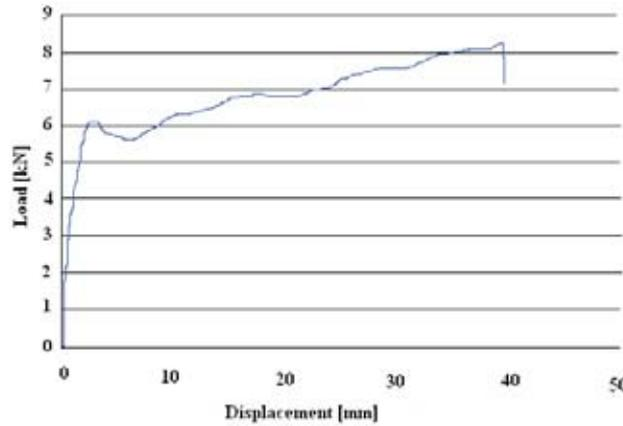
Fig. 4. Experimental results for the one-axial compression test
