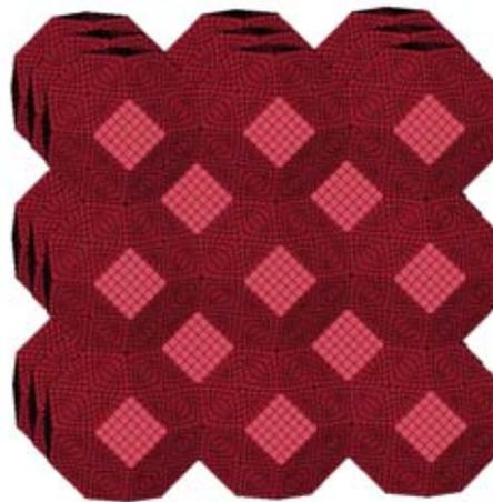
Fig. 5. Closed cell foam microstructure model
